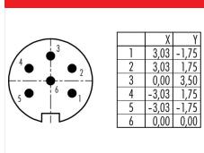
Contact arrangement (Plug-in side)
